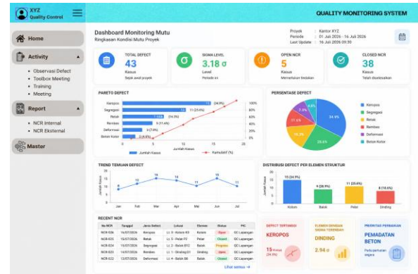
Gambar 12 Model Konseptual Dashboard Monitoring Mutu berbasis NCR
