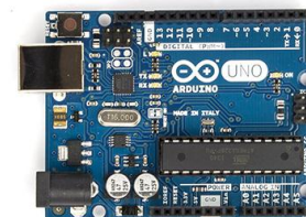
Gambar 3.1 Mainboard Arduino board model UNO R3
