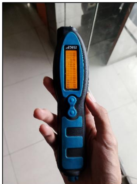
Gambar 2. Alat Pengukur Getaran - SKF Machine Condition Advisor CMAS 100-SL
